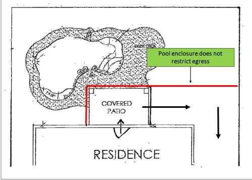
A door from the home does not open into the pool enclosure or is permanently locked or barricaded with no key accessible to a child.
